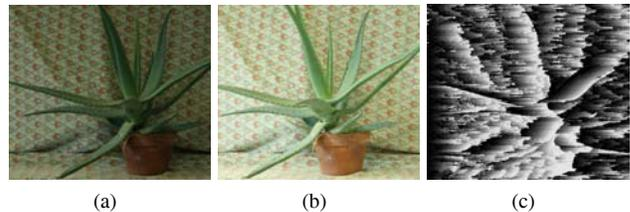
**Fig. 1.** Stereo matching of the ‘Aloe’ images under varying radiometric conditions [1]: (a) the left view with exposure level 1, (b) the right view with exposure level 2, and (c) the resulting disparity map.
