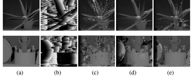
**Fig. 5.** Comparison of the disparity maps for the ‘Aloe’ and ‘Baby3’ datasets under different exposure conditions: (a) ground truth, (b) SAD [1], (c) ANCC [7], (d) ACT [5], and (e) the proposed algorithm. In this test, the exposure levels for the left and the right images are 0 and 2, respectively.
