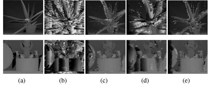
**Fig. 6.** Comparison of the disparity maps for the ‘Aloe’ and ‘Baby3’ datasets under different lighting conditions: (a) ground truth, (b) SAD [1], (c) ANCC [7], (d) ACT [5], and (e) the proposed algorithm. In this test, the lighting levels for the left and the right images are 1 and 3, respectively.
