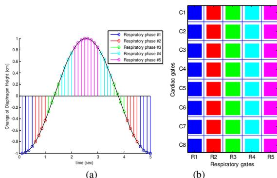
Fig 1. (a) A respiratory cycle is divided into into 40 equally spaced time intervals and 10 equally-spaced respiratory phases. The respiratory phases are paired into 5 gates according to the amplitude of the diaphragm height; (b) the respiratory-cardiac intervals are arranged into 5 respiratory and 8 cardiac gates.
