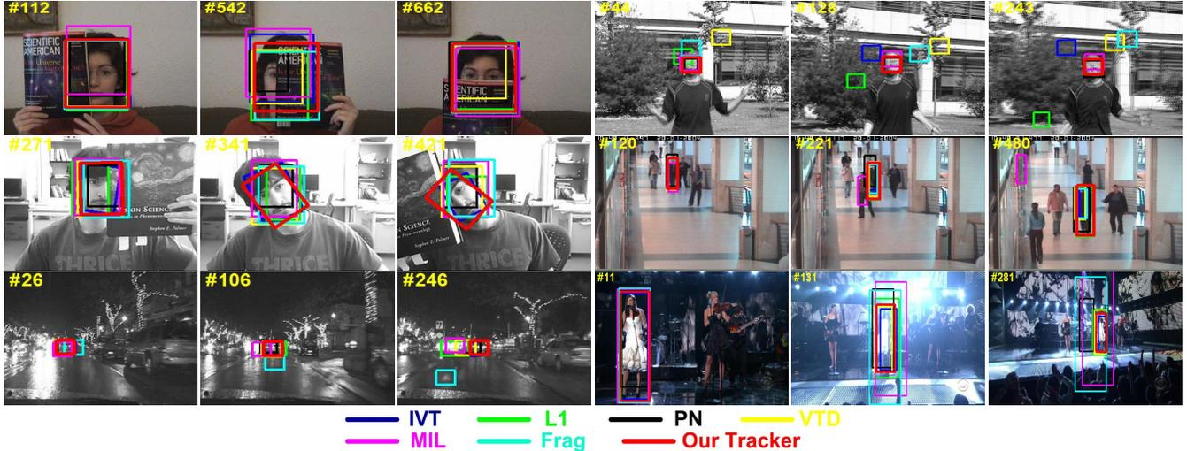
**Fig. 2.** Qualitative comparison with six state-of-the-art trackers. From left to right, the first row is *Occlusion1* and *Jumping*, the second row is *Occlusion2* and *Caviar2*, the third row is *Car11* and *Singer1*.
