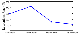
Fig. 5. The recognition rates for different THD orders.
